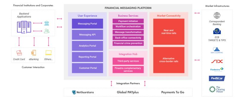
In addition to Swift, Finastra Financial Messaging can provide connectivity to many other market infrastructures and PSPs, allowing customers to manage these services in a consistent manner and determine service routing at an enterprise level.
